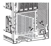
3 Install the HDD cage.
